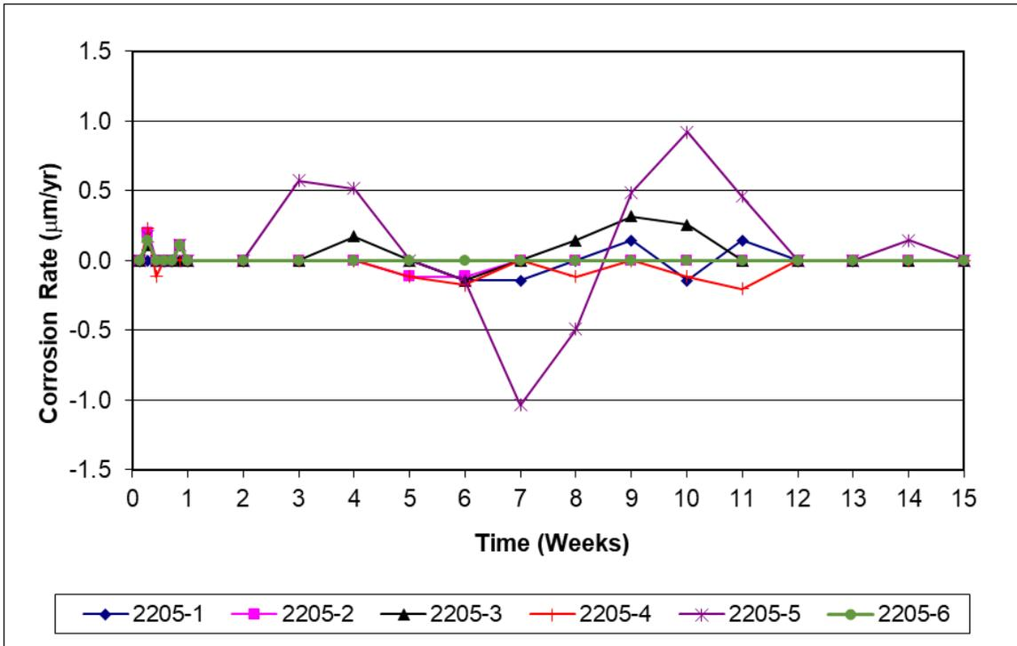
**Figure 3:** Individual corrosion rates ( $\mu\text{m}/\text{yr}$ ) for 2205 stainless steel.
