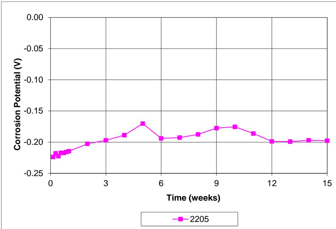
**Figure 5:** Average corrosion potential (vs. CSE) for 2205 stainless steel.
