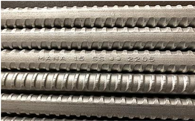
**Figure 1:** 2205 reinforcing steel evaluated in this report.
