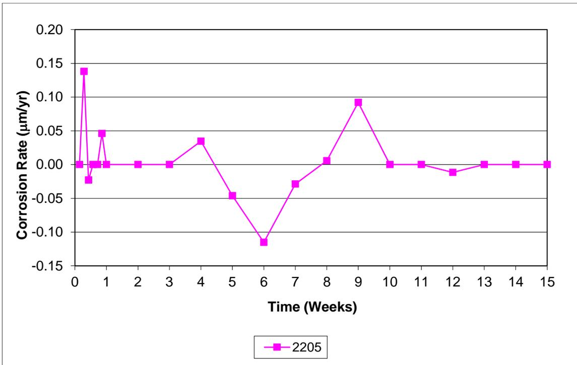
**Figure 5:** Average corrosion rates ( $\mu\text{m}/\text{yr}$ ) for 2205 stainless steel.
